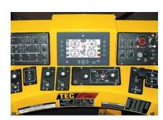
The new TEC® Plus electronic control system features CAN bus technology, which utilizes multiple control modules located throughout the machine for real time performance data and advanced troubleshooting capabilities.
