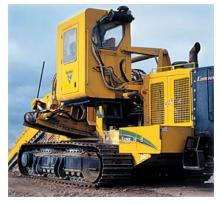
A 600 hp (447 kW) Caterpillar Tier 3 engine delivers the power needed to triumph over tough rock-trenching projects.
