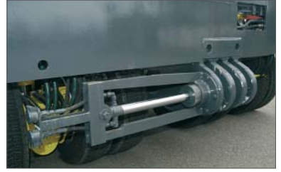
On request: hydraulic bolting device
