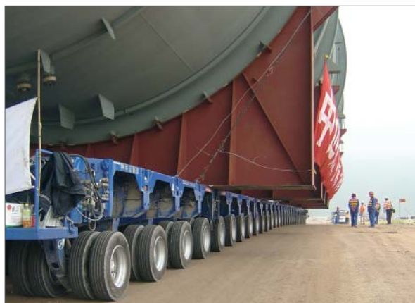
The large axle compensation guarantees uniform load distribution
