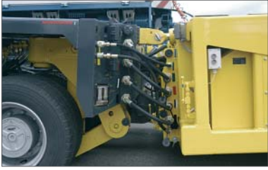
Connection of hydraulics and electronics through quick-release couplers
