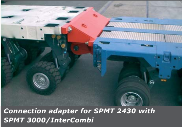
Combination of SPMT 2430 with SPMT 3000/InterCombi
