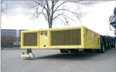
Power Pack Unit provides power for drive, lift and steering
