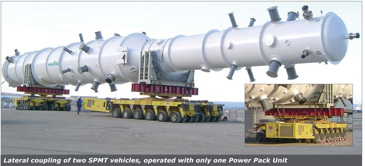
Connection adapter for SPMT 2430 with SPMT 3000/InterCombi
