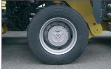
Hydrostatic wheel drive in the twin-tyred pendulum axles
