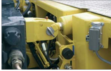
Centering actuator for raising and lowering of the Power Pack Unit
