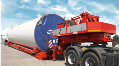
Wind tower segment on a frame deck
