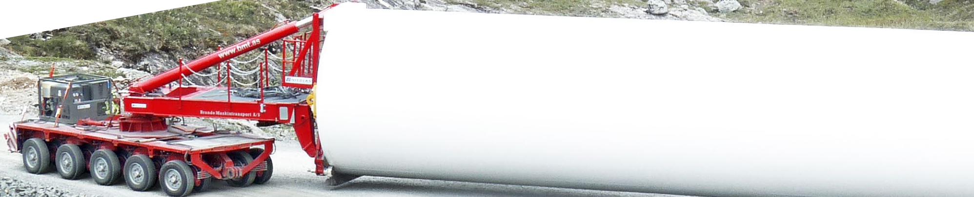
Wind tower bolster on a K25 H
