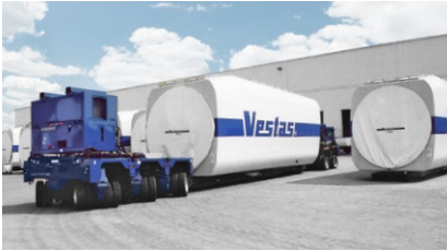
Vestas nacelle on a SCHEUERLE InterCombi SP
