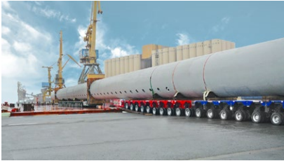
K25 H SPE transporting a monopile
