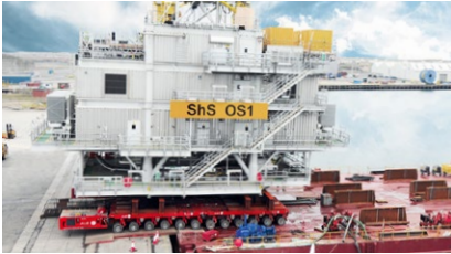
SPMT of SCHEUERLE with an off-shore transformer station driving onto the ship
