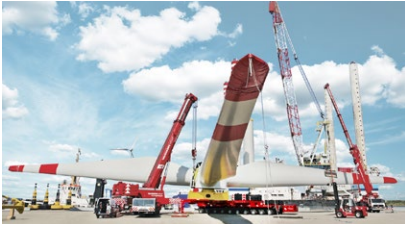
Transport of an entire off-shore rotor blade assembly
