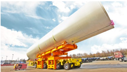
Wind tower bolster on a K25 H
