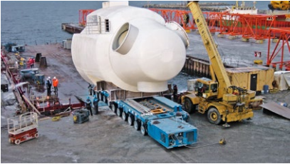
KAMAG K24 in action: an off-shore wind turbine with hub rolling onto a pontoon
