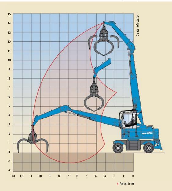
Work equipment: box-type boom 7.85 m (25.8'), dipperstick 4.5 m (14.8')
