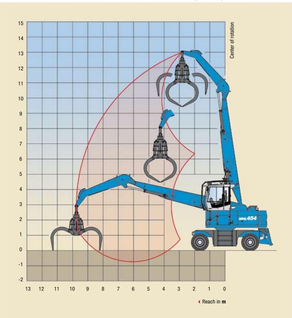
Work equipment: box-type boom 7.1 m (23.3'), dipperstick 4.1 m (13.5')
