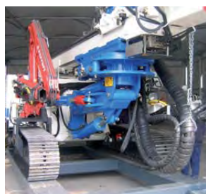
Std. kinematic articulation 4x90° sector turntable
