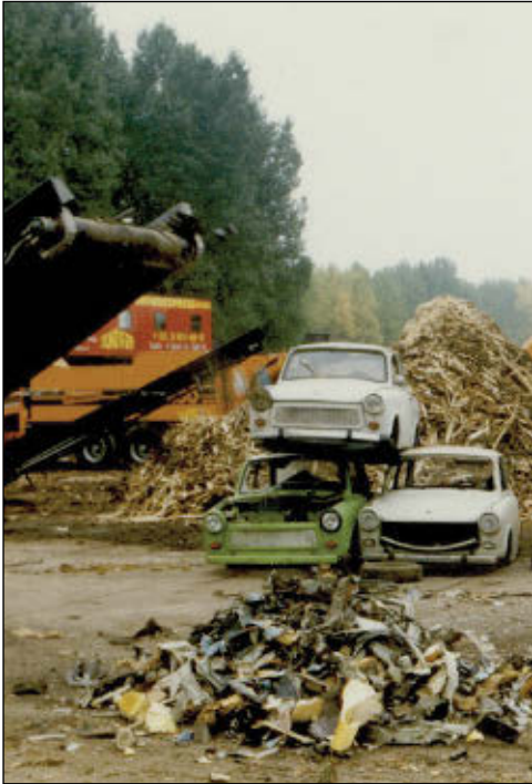
Doppstadt DL 150 Shredder Volume reduction of a Trabant car body
