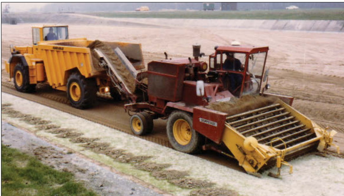
Doppstadt FBRM 2800 (filter basin cleaner) Converted from the basis of a field cropper machine
