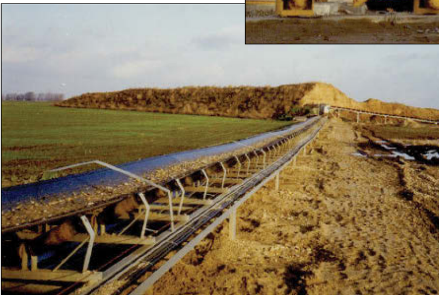
Doppstadt Belt Conveyor Sleewable stockpiling conveyor
