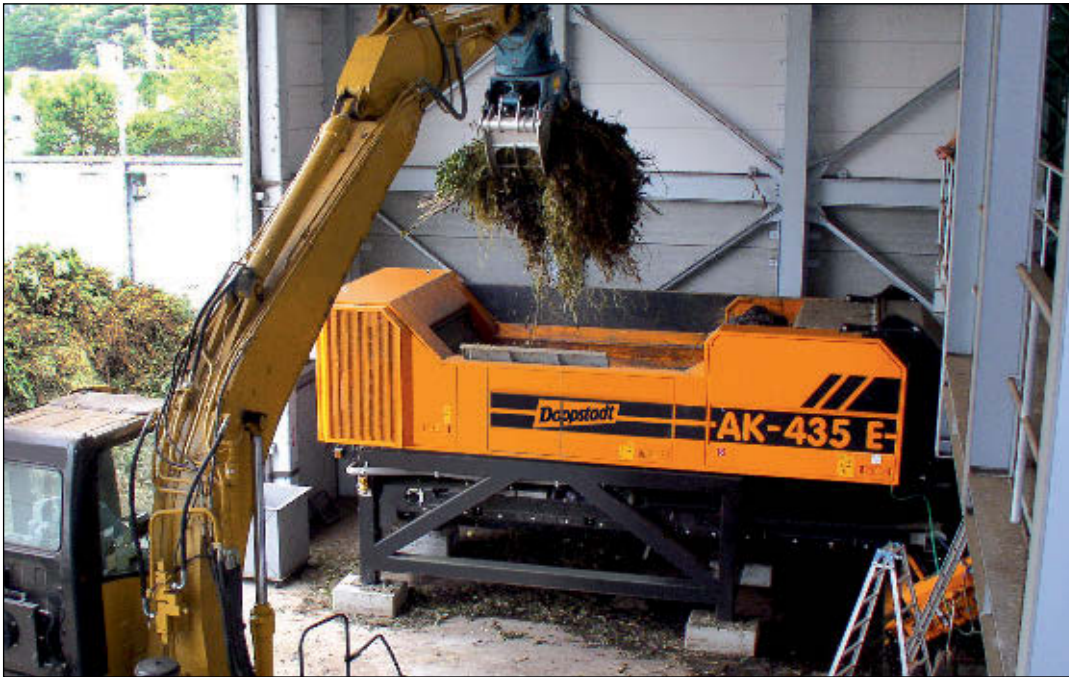
Doppstadt Grinder AK 435 E Static machine with AC engine
