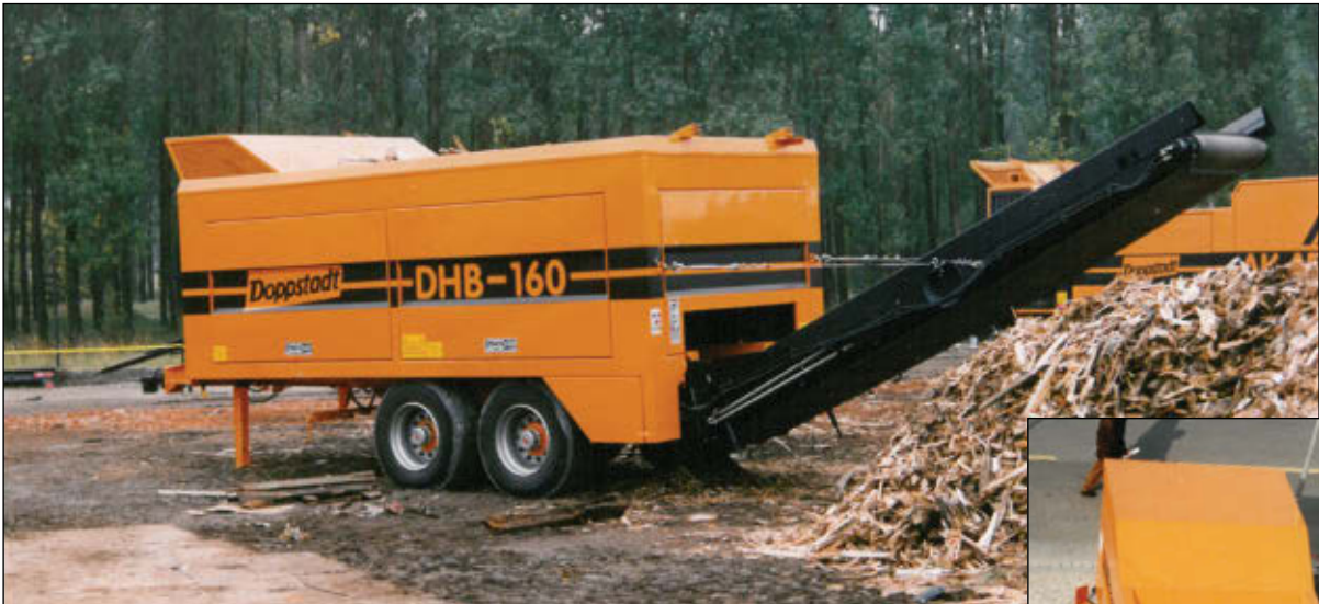
Doppstadt Shredder DHB 160 (Doppstadt wood crusher), 2-shaft shredder
