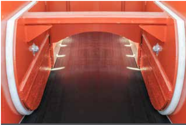
ADJUSTABLE FLOW GATE CONTROLS RATES
