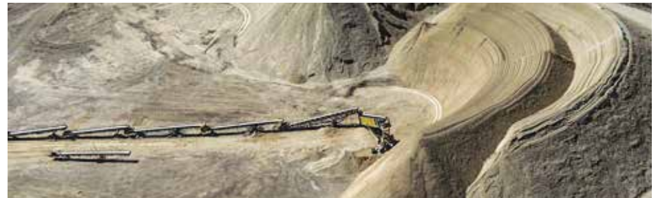
RADIAL WINDROW STOCKPILING ACHIEVES IN-SPEC MATERIAL MIX
