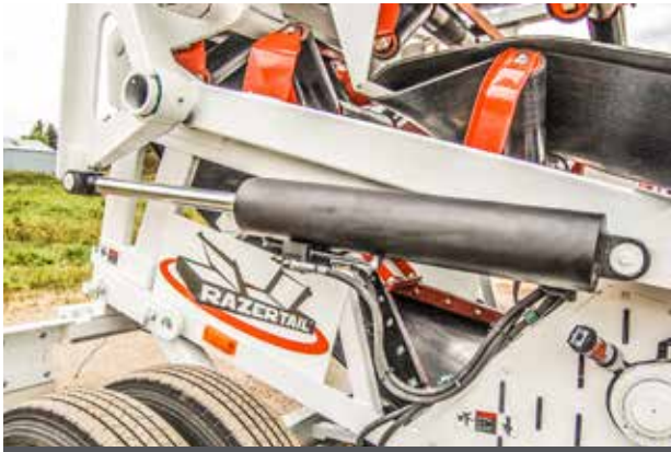
CYLINDER RODS PROTECTED DURING OPERATION
