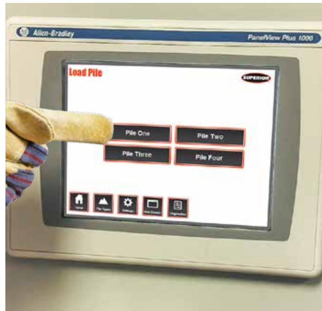
RECALL 1 OF 4 PREVIOUSLY SAVED PILE TYPES
