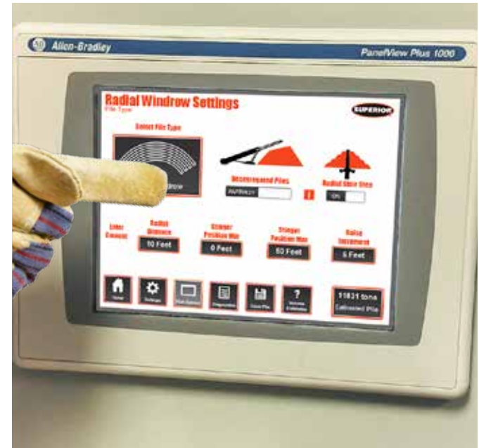
SET PILE PARAMETERS IN VISUAL SETTING SCREEN
