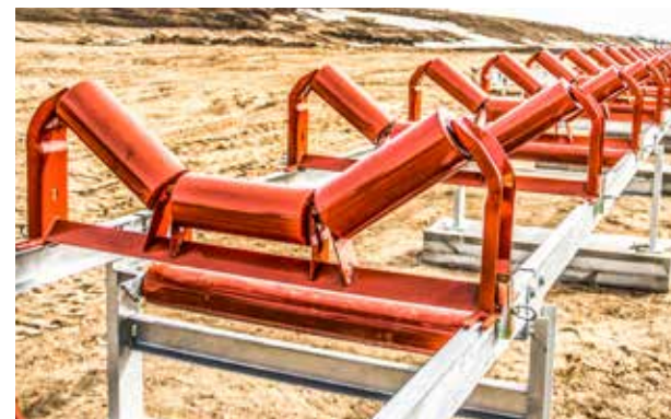
TROUGHING IDLERS ATTACH WITH J-BOLTS
