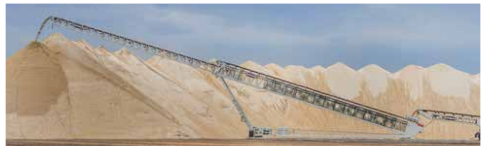
A 190' TSSA IS CAPABLE OF PRODUCING A 209,300 CUBIC YARD STOCKPILE
