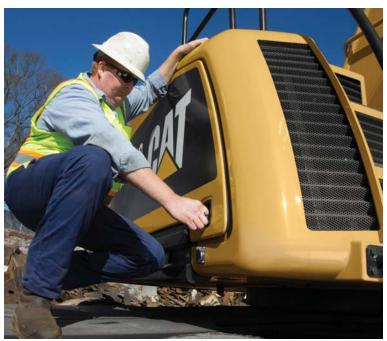
To ease serviceability on the MH3049, all primary service points are conveniently located under a single access service panel on the right side of the machine or beneath the top engine access panel. Easily locate components with the engine and cooling system's longitudinal layout. Both panels are hinged with gas struts, ensuring that one technician can easily access all maintenance points.
