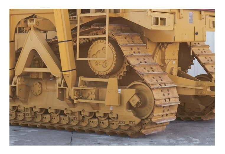
**Final Drives.** Final drives and associated power train components are raised above the work area, isolating them from ground induced impact loads, as well as pipelayer loads, extending power train component life.
