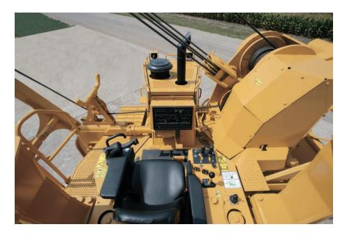
**Clear Full-Circle View.** A tapered hood and "notched" fuel tank give the operator a clear line of sight to the front, rear and side work areas. The new streamlined design of the Caterpillar 583T Pipelayer offers several operator visibility improvements for more precise maneuvering and placement of pipe.
