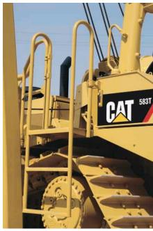
**Access Ladder.** Direct access to the operator's station utilizing ladder on left side of the machine.
