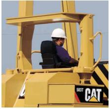
**Optional Rollover Protective Structure.** Provides increased operator protection.
