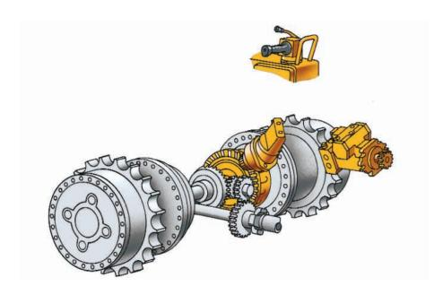
**Differential Steering System.** A planetary differential turns the machine by speeding up one track and slowing the other, while maintaining full power to both. The system consists of three planetary gear sets.
