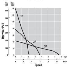
**Drawbar vs. Speed.** As loads on the tractor increase, the 583T offers unmatched lugging capability and smooth shifting as the need occurs to change gears under varying loads. The 3-speed forward, 3-speed reverse transmission, backed by differential steering, offers excellent runout speeds and accurate steering capability under load.
