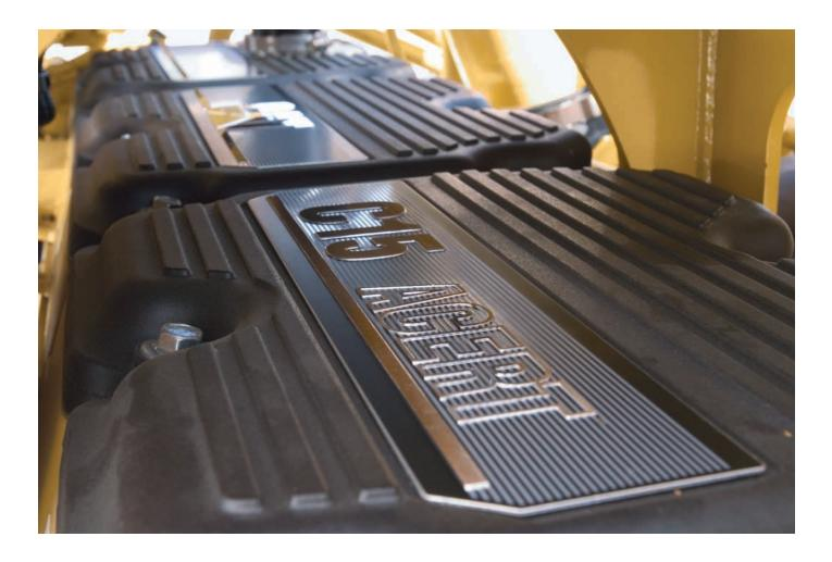
**Engine.** The Cat C15 engine with ACERT<sup>TM</sup> Technology provides the power for the 583T. Performing at full-rated net power of 231 kW (310 hp) at 1,850 rpm, the large displacement and high torque rise provides the 583T the power needed on challenging jobs. Matched to the high-efficiency torque divider and electronically controlled power shift transmission, it will provide years of dependable service.
