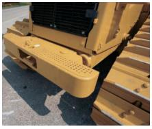
**Front Bumper.** A front bumper is pinned on the frame rails and provides both protection and a towing device. Pipelayer frame mounts are also an integral part of the frame.
