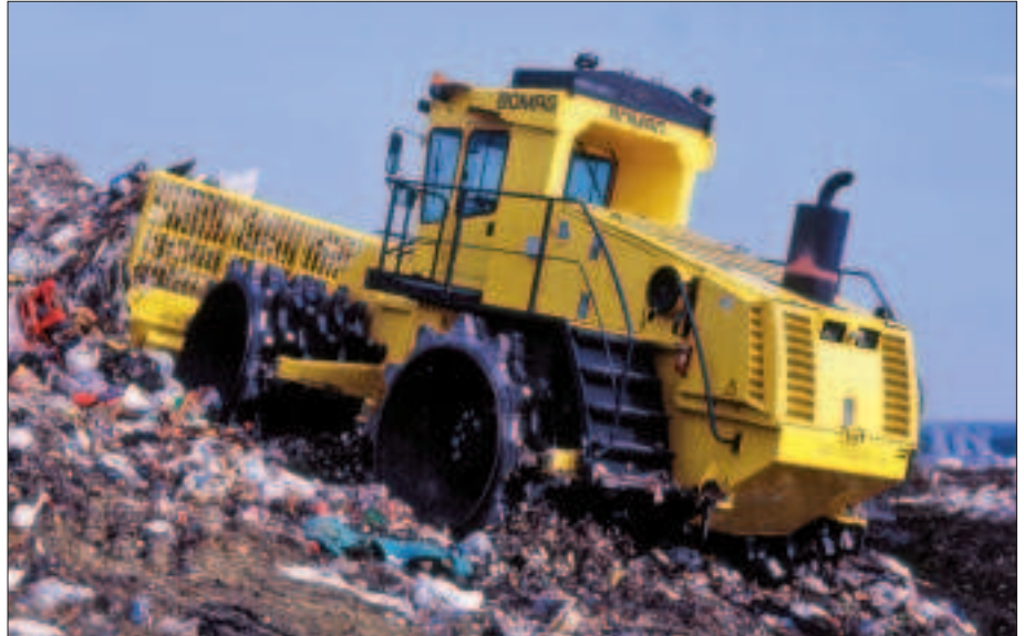
4-wheel hydrostatic drive system is capable of 100% gradeability, 45° slopes
