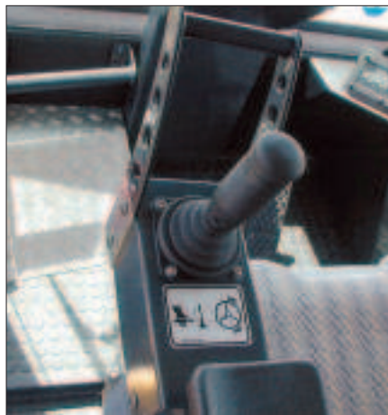
Ergonomic control layout including joystick steering control.
