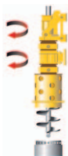
Cased Kelly drilling (installation with BTM)
