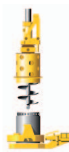
Cased Kelly drilling (installation with oscillator)
