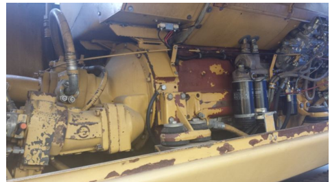
Deutz Diesel - engine with hydraulic pumps
