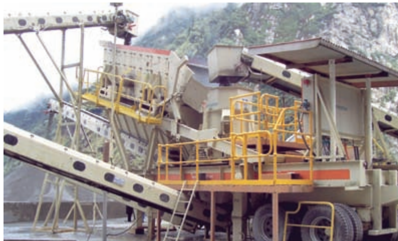
NW7100C, a portable Barmac plant with an inclined screen.
