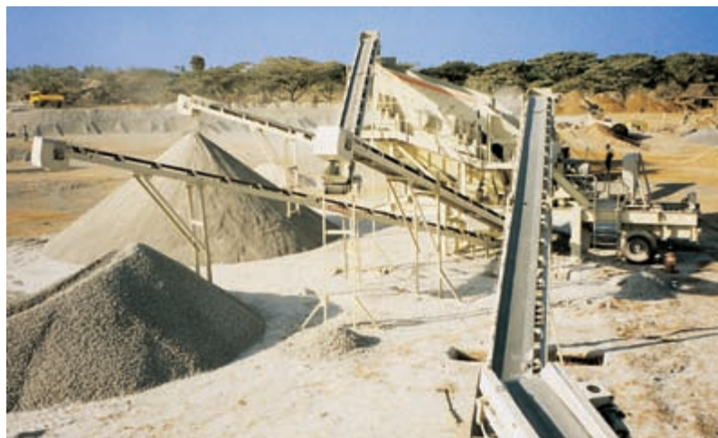
Two stage portable crushing and screening process in India with NW80 jaw plant and NW100GPC cone plant.
