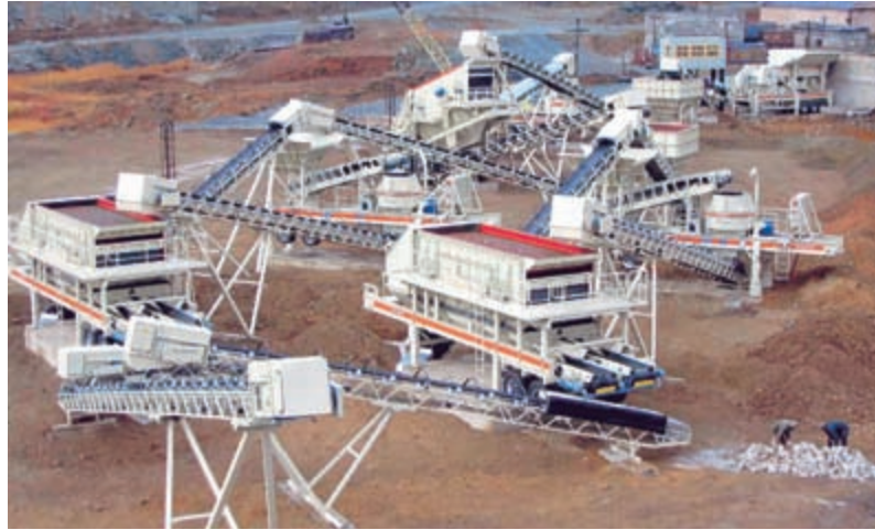
Complete crushing and screening process in Kazakhstan built with four portable crushig plants and three portable screens.
