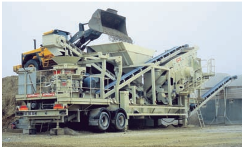
Nordberg NW100HPC-CC, working in France, is built around a HP100 cone crusher.
