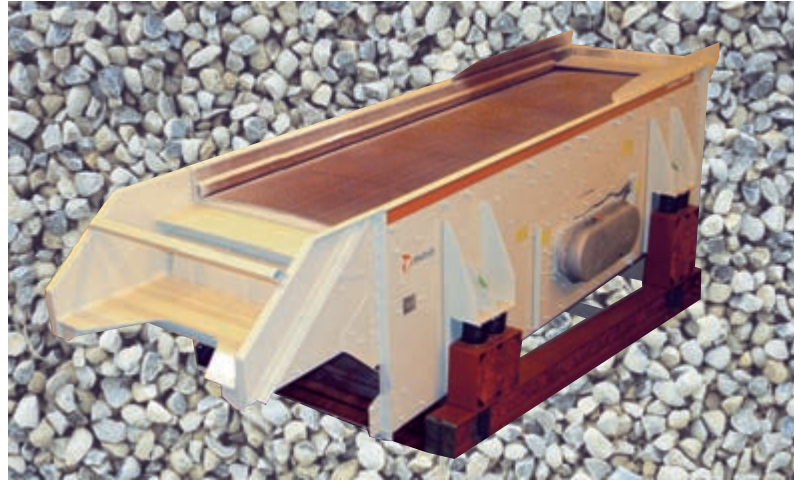
Nordberg FS screens are built of modular components assembled with huck bolts which decrease any failure risk due to fatigue stress.
