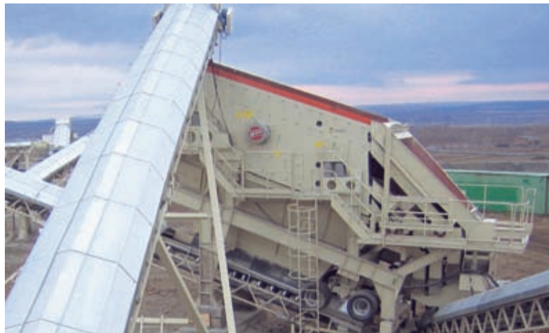
NW Series screen plant equipped with CVB2060-4 inclined screen working in Kazakhstan.
