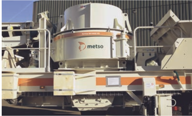
Barmac B Series vertical shaft impactor is the original rock-on-rock VSI crusher.
