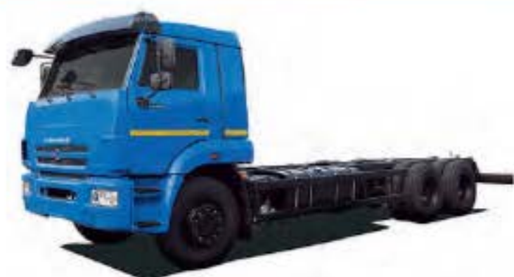
Dimensions with curb (gross) weight 4910+1440 mm wheelbase is used in modifications with the rear air suspension
