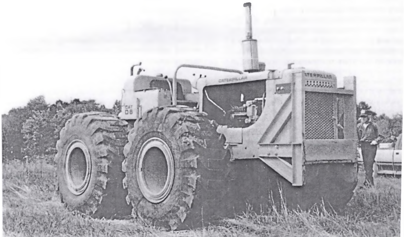
Caterpillar DW6. Caterpillar also offered its D4 and D6 tractors as wheeled options. The DW6 was offered as far back as 1952 when about 100 of the then-current 9U D6 were built for sugar cane operations. Beginning in 1962, up to 200 DW6 tractors were produced based on the 44A Series D6, which replaced the 9U Series in 1959. The engine in those machines was rated at 115 flywheel-horsepower. The example is shown fitted with a push block and double-drum rear winch for pulling scrapers. Keith Haddock
