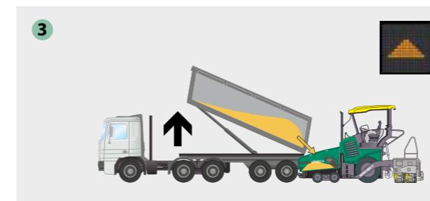
Raise Dump Box: Lorry raises the dump box.
