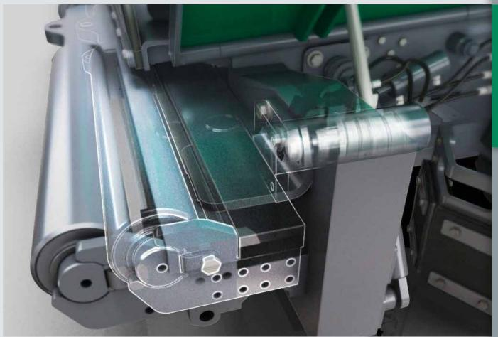
**Especially wide** and oscillating push-rollers support convenient, shock-free docking of feed vehicles.
