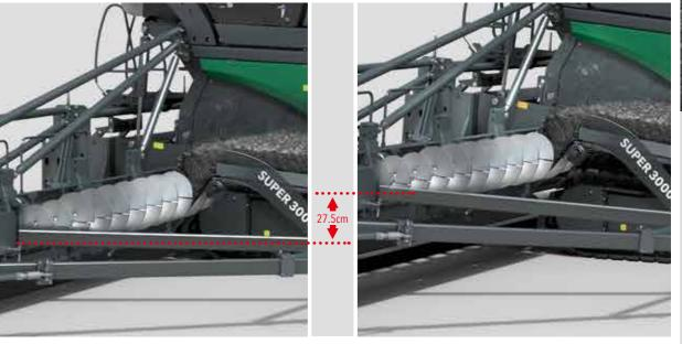
Innovative material handling concept in which the height of the conveyor and auger can be jointly adjusted. This optimizes the supply of mix even when paving thick layers of up to 50cm. Optimum transfer of mix to the auger at all layer thicknesses thanks to the infinitely height-adjustable chassis.
