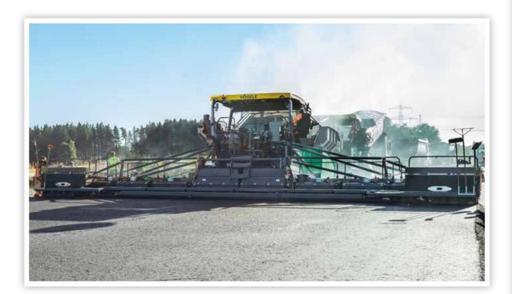
With a pave width of up to 18m, a maximum laydown rate of 1,800t/h and an engine output of 354kW, the SUPER 3000-3 is the new flagship in VÖGELE's paver line-up. As a representative of the Premium Line, this large paver incorporates all the features of the "Dash 3" generation.
