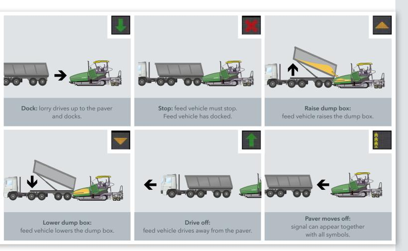
PaveDock Assistant is the communication system between the paver operator and the driver of the feed vehicle. It allows particularly fast and reliable transfer of mix to the paver. Signal lights on the paver and the associated controls on the paver operator's ErgoPlus 3 console are key components.
