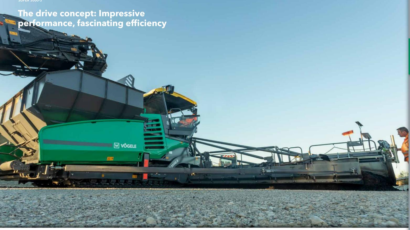
**The powerful 6-cylinder diesel engine** rated at 354kW is the driving force behind the Highway Class paver.
