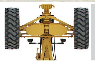
Front axle steering cylinder has been designed to enhance durability and hydraulic hoses have been routed to improve reliability.
