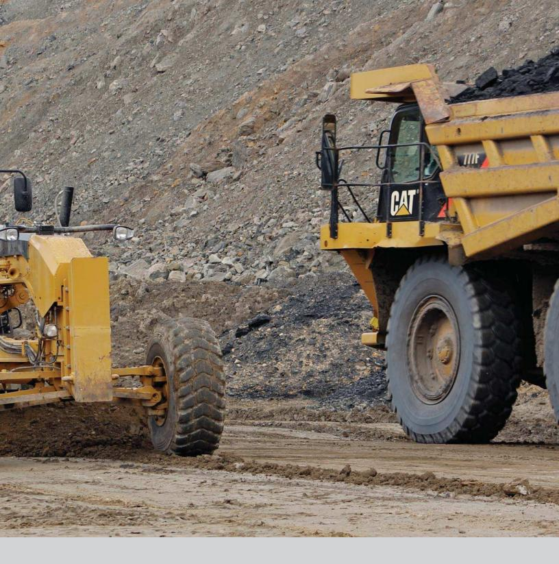
With additional power, wider moldboard and the possibility to use a more aggressive blade angle; the 18M3 enhances operational efficiencies by increasing coverage and reducing the number of passes required to grade your haul roads.
