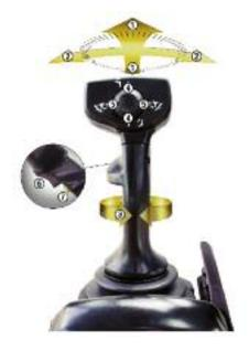
**Right Joystick Functions.** The right joystick primarily controls the Drawbar, Circle and Moldboard functions.
