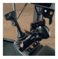
**1 – Ripper Control Pod.** Infinitely variable roller switches control the rear ripper and/or front lift group (when equipped), for easy and comfortable control.
