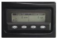
**Cat Messenger.** Standard on the 16M, Cat Messenger provides real-time machine performance and diagnostic data with an easy-to-use interface. Messenger monitors all system data and alerts the operator of any faults through a digital text display that can be shown in multiple languages.
