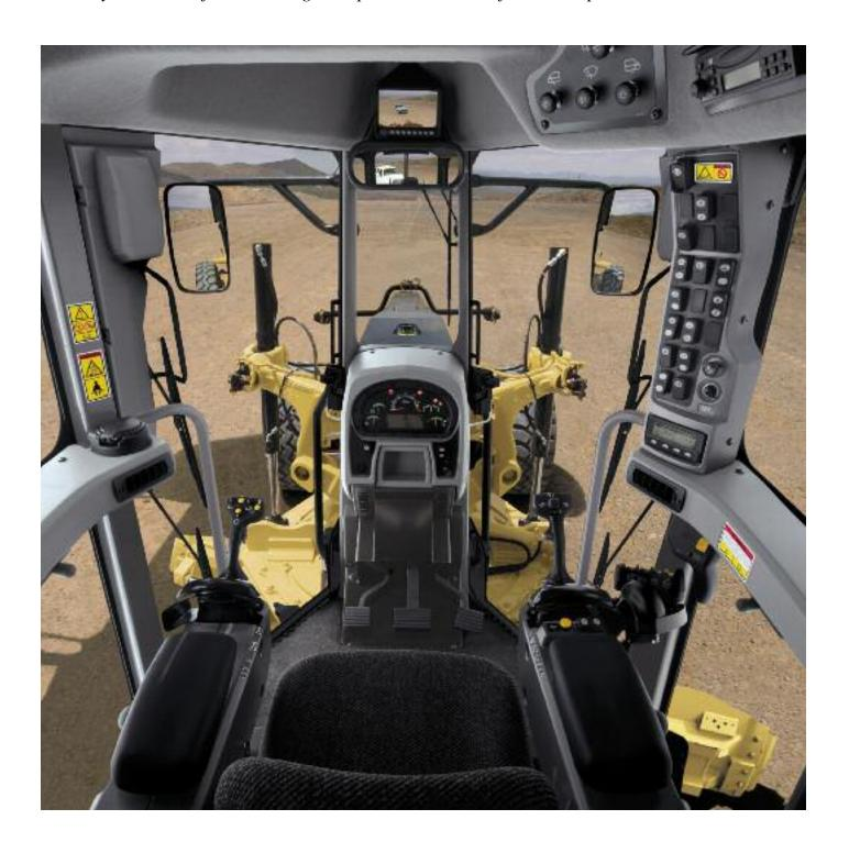
**Advanced Joystick Controls.** Two electrohydraulic joysticks reduce hand and wrist movement as much as 78% compared to conventional lever controls for greatly enhanced operator efficiency. The intuitive pattern is easy to learn and provides the precise implement control you expect from Caterpillar.
