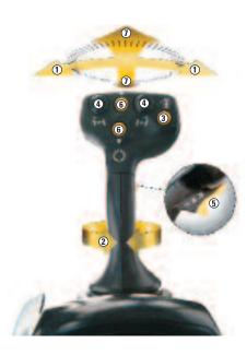
**Left Joystick Functions.** The left joystick primarily controls the machine direction and speed.
