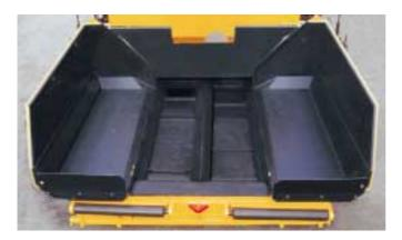
Individual hydrostatic drives for each conveyor and each distributor auger:
