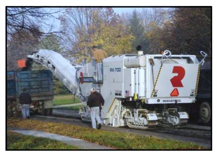
The RX-700 is a 700 horsepower cold planer available with either three or four track assemblies. This versatile machine allows contractors to cut up to 14" (35.6 cm) deep with widths of 6'7" (2 m), 7'2" (2.184 m). The RX-700 offers contractors more versatility and productivity. A 36" inch front load-out conveyor, with 60° swing to either side, provides ample loading capacity.
