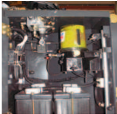
Central lube system reduces maintenance time
