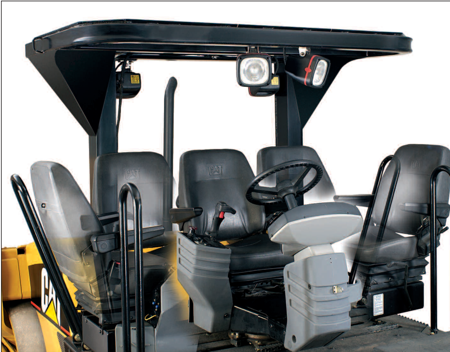
For FOPS protection to be effective, the operator must be seated under the canopy.
