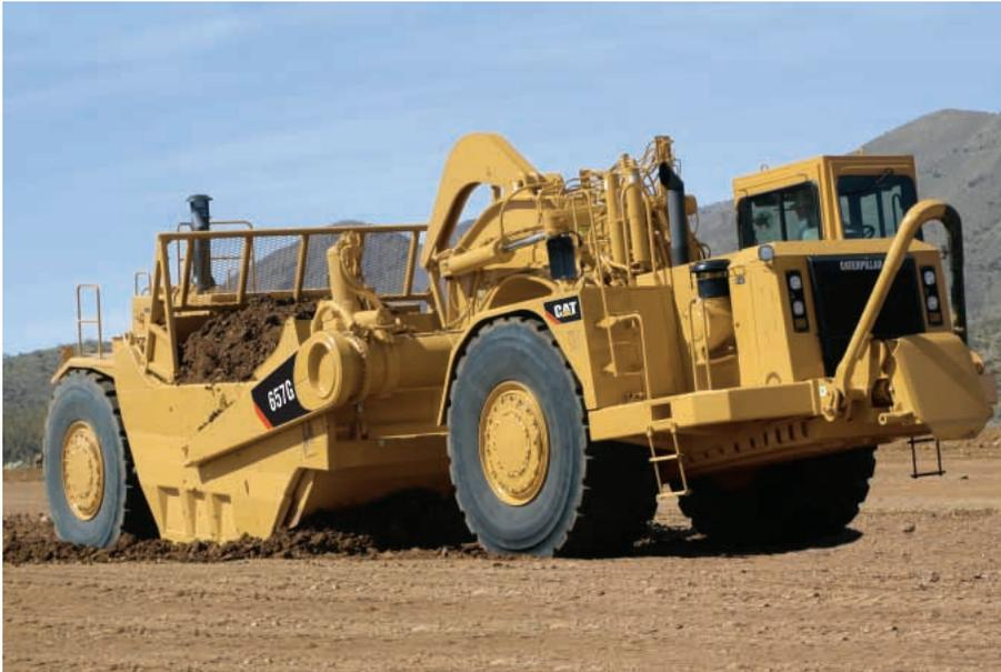
**Redesigned Bowl.** The redesigned bowl minimizes falling material lodging between the bowl and the draft arm, resulting in premature wear. The modifications also provide better load retention on level ground or traversing down a grade.
