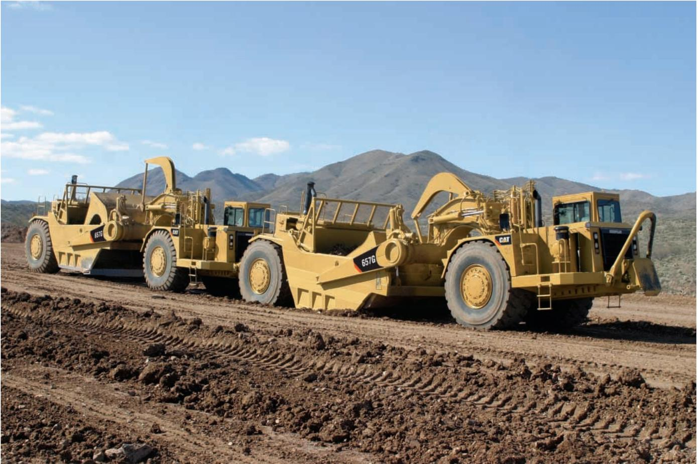
**Push-Pull Attachment.** This optional arrangement concentrates the combined horsepower of two machines onto one cutting edge. The push-pull attachment allows two individual machines to act as a self-loading system, typically loading both machines in less than a minute.
