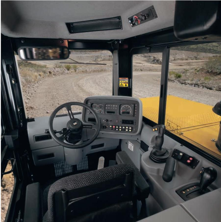
**Seat Suspension.** The new standard seat suspension features a high performance air shock absorber with a self-contained air compressor. For operators requiring additional damping, dual shock absorbers in the seat suspension are available.
