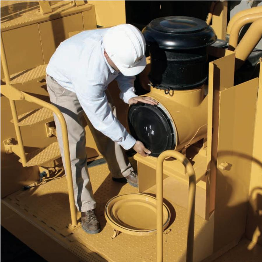
**Grouped Service Points.** Maintenance and service points for the engine are grouped on the right-hand side for easy access. They include the engine air cleaner, engine oil check and fill, fuel filters and priming, coolant level sight glass, window washer bottle, air conditioning dryer cartridge, ether starting aid canister, engine oil filter, fan drive lubrication, and sampling ports for the engine oil and coolant.
