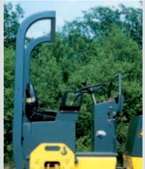
Vibration isolated operators platform makes driving fatigue-free
