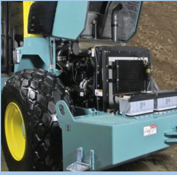
Accessible engine compartment and battery location
