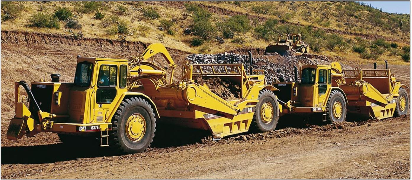
**Wide cutting edge** scoops large volume loads from shallow cuts, while the low-profile design of the bowl offers less resistance to incoming materials.
