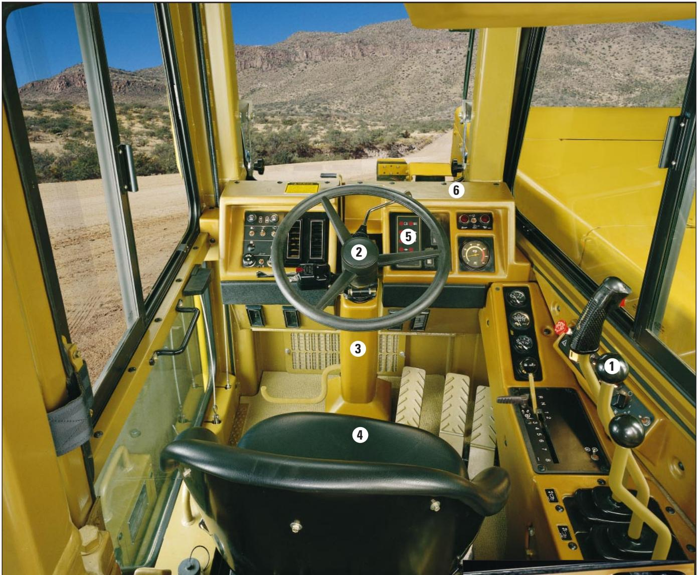
**Standard rubber-mounted cab** reduces noise and vibration for comfortable, shift-long operation.
