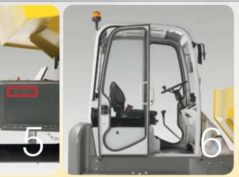
4 The tidy, robust cockpit extends over the full breadth of the chassis. It protects the
