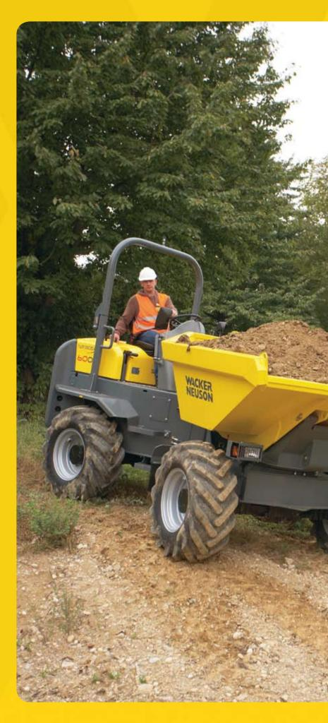
Payload 3,000 kg: The Wacker Neuson All-wheel dumper 3001.
