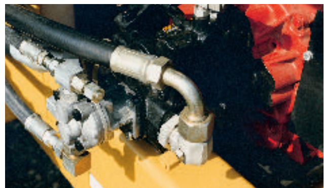
Piggy back gear pump provides priority flow for steering.
