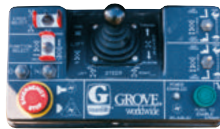
Convenient removable control box features patented enable button.
