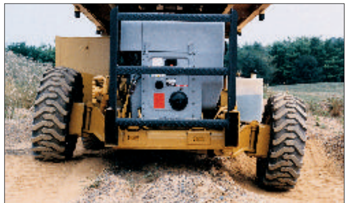
Oscillating rear axle is optional.
