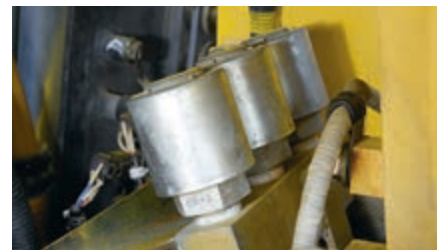
Canister-type breathers facilitate checking and cleaning (optional)
