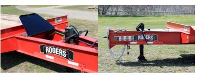
■ Longer drawbar & premium landing gear: Longest drawbar in the industry makes for better load distribution and easy handling. 1/2" safety chains are integral to the frame of the trailer, not welded or bolted in place. The two-speed landing gear has 50,000 lb. lift capacity and 70,000 lb. static capacity. The pintle eye adjusts to accomodate various heights using standard shop tools. There is ample room for chain and tool storage in the drawbar toolbox with lockable steel lid.
