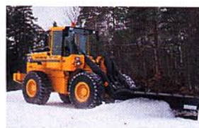
Snow blade For snow clearance. Hydraulically adjustable.
