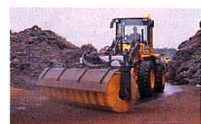
Sweeper Sweeper for connection to attachment bracket. Can be equipped with water tank and spray nozzles.
