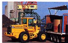
Hydraulic bale clamp Equipment for efficient handling of e.g. bales and reels.
