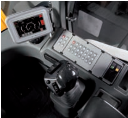
Liebherr operating lever, with electro-hydraulic pre-control
