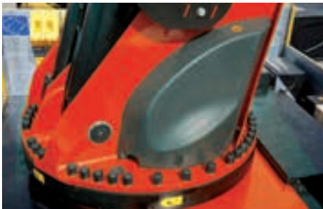
CONTINUOUS SLEWING SYSTEM UNRESTRICTED MOVEMENT
