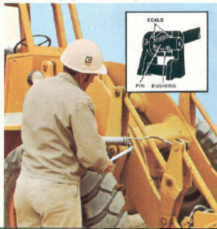
Loader linkage greased from ground
