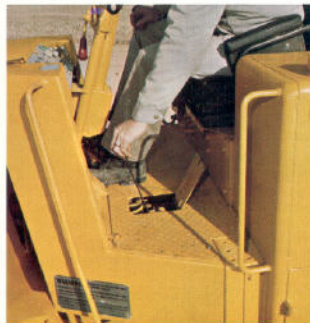
Loader linkage greased from ground
