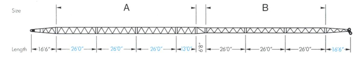
Blue figures: elements alternatively used for either lattice boom extension or luffing jib configuration.
