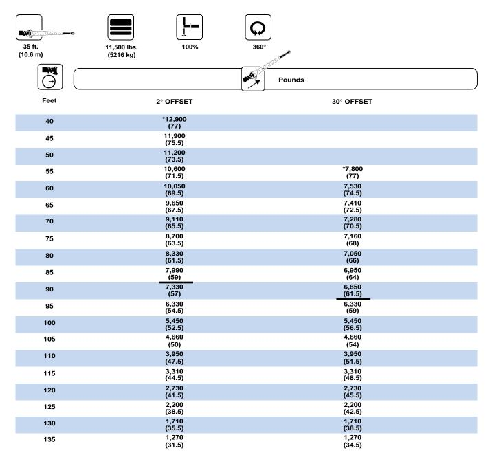
NOTE: () Boom angles are in degrees. \*This capacity is based upon maximum boom angle.
