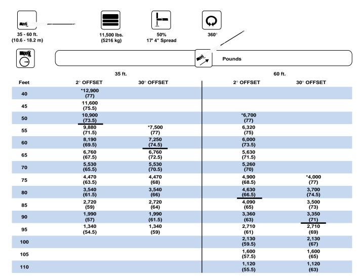
\*This capacity is based upon maximum boom angle.
