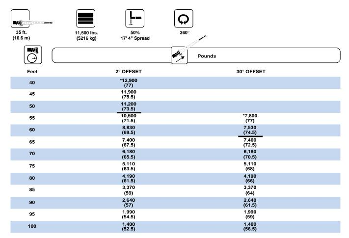
NOTE: () Boom angles are in degrees. \*This capacity is based upon maximum boom angle.
