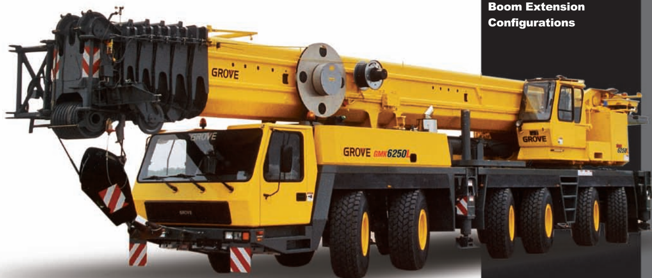
All Terrain Crane
