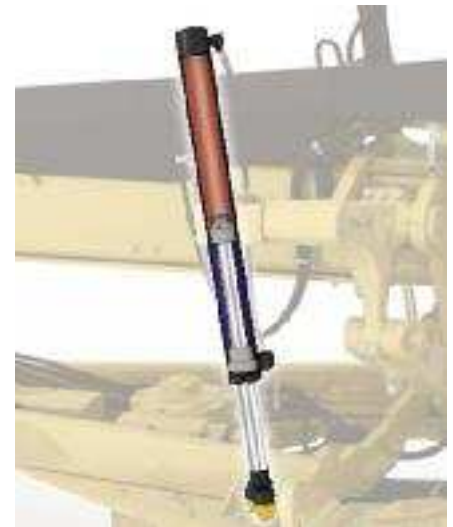
Blade lift cylinder: red = 40 L/min (10.6 gal/min), blue = 24 L/min (6.3 gal/min)
