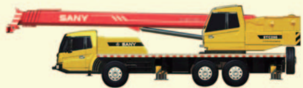
STC250H Max Rated Payload: 25t Main Boom: 5 Sections, 10.5-39.5 Extended Chassis: 6x4x2
