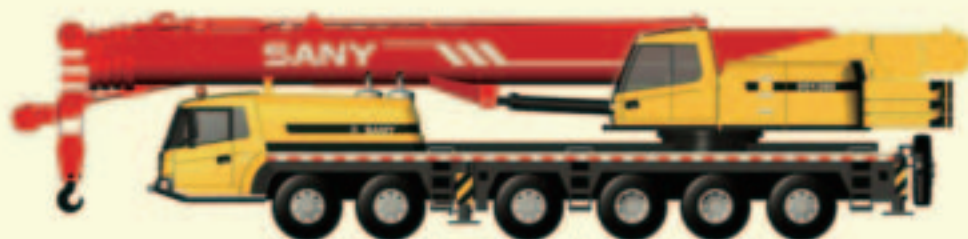
STC1300 Max Rated Payload: 130t Main Boom: 6 Sections, 13.3-60m Extended Chassis: 12x6x8
