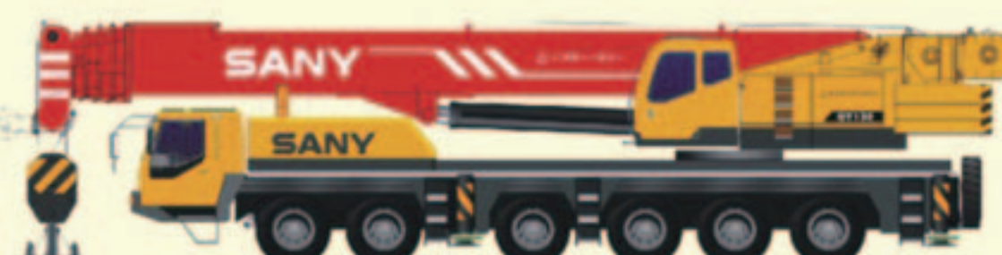
QY130 Max Rated Payload: 130t Main Boom: 6 Sections, 13.3-60m Extended Chassis: 12x6x8
