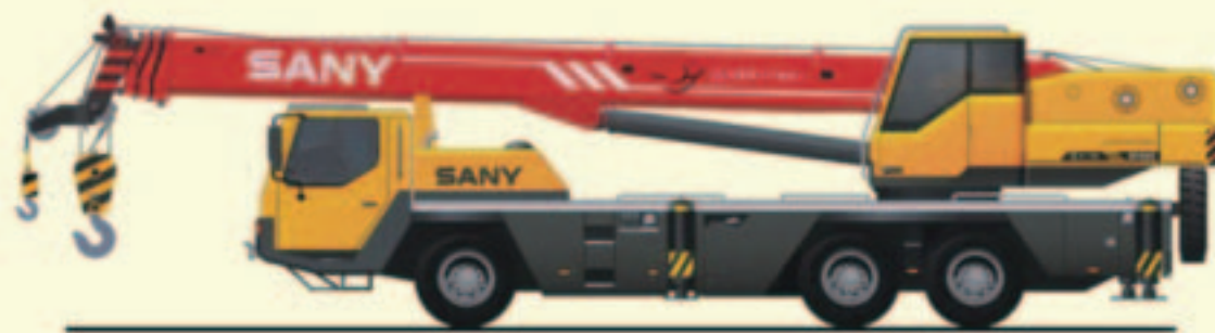
QY25C Max Rated Payload: 25t Main Boom: 4 Sections, 10.65-33.5m Extended Chassis: 6x4x2
