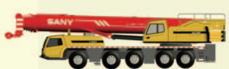
SAC1800 Max Rated Payload: 180t Main Boom: 6 Sections, 13.5-62m Extended Chassis: 10x8x10
