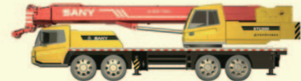
STC750 Max Rated Payload: 75t Main Boom: 5 Sections, 11.8-45m Extended Chassis: 8x4x4
