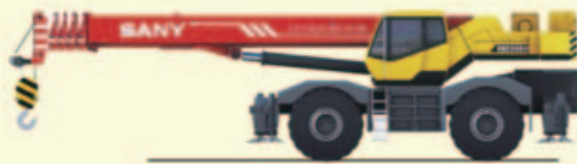
SRC550H Max Rated Payload: 55t Main Boom: 5 Sections, 11.5-42.5m Extended Chassis: 4x4x4
