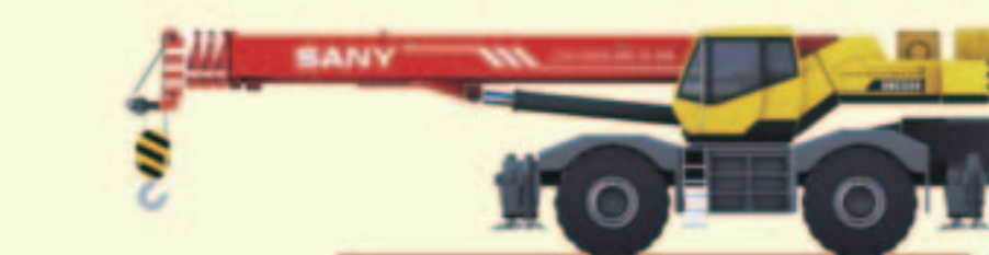
SRC550 Max Rated Payload: 55t Main Boom: 4 Sections, 11.25-34.5m Extended Chassis: 4x4x4
