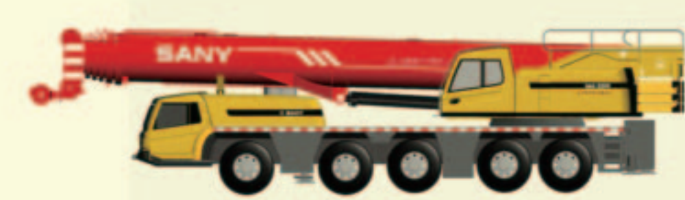
SAC2200 Max Rated Payload: 220t Main Boom: 6 Sections, 13.5-62m Extended Chassis: 10x8x10
