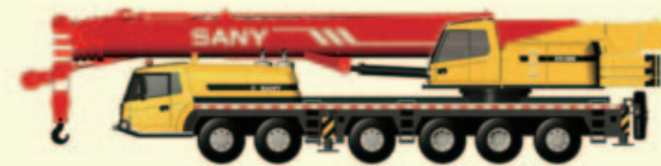
STC1000 Max Rated Payload: 100t Main Boom: 5 Sections, 13.5-52m Extended Chassis: 12x6x8
