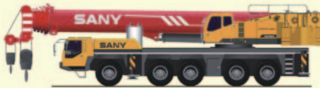
QAY220 Max Rated Payload: 220t Main Boom: 6 Sections, 13.5-62m Extended Chassis: 10x8x10
