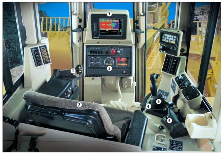
Clear working view. Angled seat, tapered hood and "notched" fuel tank give the operator a clear line of sight to the front and rear work areas. Large single-pane door windows allow the operator to see close-in to each side without leaning.
