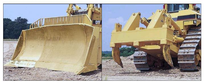
**Bulldozers.** The 11SU blade, rated at  $27.2 \text{ m}^3$  (35.5 yd³) and the 11U blade at 34.4 m³ (45.0 yd³) make full use of D11R power.
