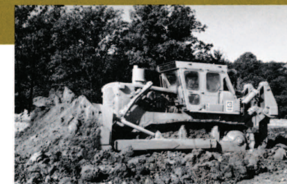
Shown with optional ROPS Modular Cab, track roller guards, lights, hydraulic control, 9S Bulldozer and single shank ripper.
