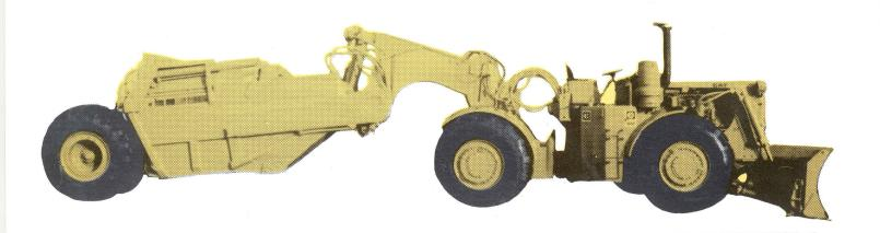
THE CATERPILLAR 830 M IS A FOUR-WHEEL DRIVE, ARTICULATED TRACTOR WITH THE POWER AND WEIGHT FOR PRODUCTION DOZING PLUS THE SPEED AND MOBILITY NECESSARY FOR TRANSPORT ASSIGNMENTS.
