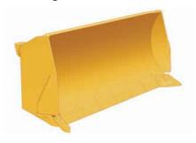
**Heavy-Duty Semi-U Blade.** Utilizes the same design as the standard Semi-U blade with the addition of a Hardox 400 liner plate, Hardox material on the side plates and additional gusseting on the bottom of the blade provide increased strength and durability in high wear applications.
