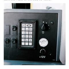
**Rimpull Control System.** Has four factory preset rimpull settings (low, medium, high and maximum) to better match ground conditions.
