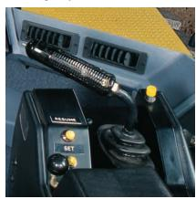
**Blade Control.** Floor-mounted controls adjust lift/lower and tilt/tip blade functions. (2)
