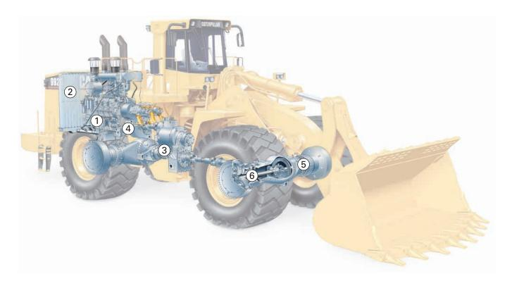
**Cat 3508B Diesel Engine.** Is a four-stroke design and uses long, effective power strokes for more complete fuel combustion and optimum efficiency. (1) It is designed with large displacement and a low speed rating for long hours of service between scheduled overhauls and lower operating costs.
