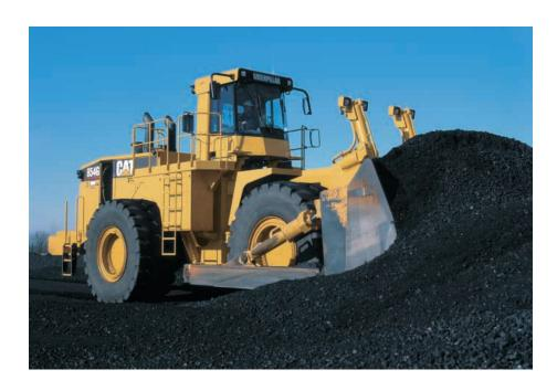
**Heavy-Duty Blade Linkage.** Is common with the Caterpillar D11 Track Type Tractor. These well-proven components are designed for large dozing loads in tough applications.
