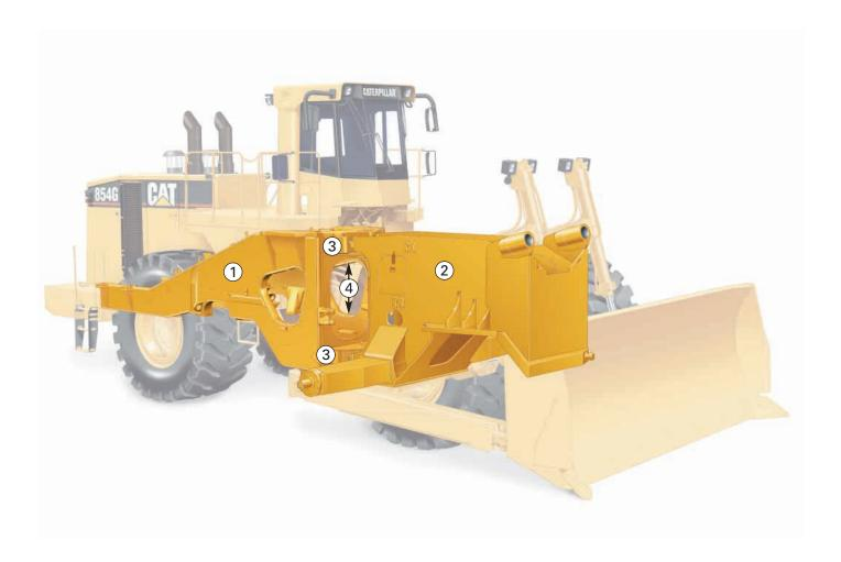
Castings. In the engine end frame are used in critical high-stress areas to help spread the load and reduce the number of parts. The casting for the rear trunnion mount also serves as an engine mount, which provides a load path for the weight and torque of the engine to travel down to the trunnion and then on through to the axle. Other castings used in the engineend frame include: front trunnion mounts, steering cylinder brackets, articulation stops and lock link.
