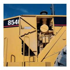
**Swing-out Doors.** On both sides of the engine compartment provide easy access to the engine oil dipstick and filler spout, fuel filters, air conditioner compressor, engine oil filters, alternator, starting receptacle, air filter service indicator, coolant fill and ether starting aid. The disconnect switch and diagnostic connector are located on rear platform.
