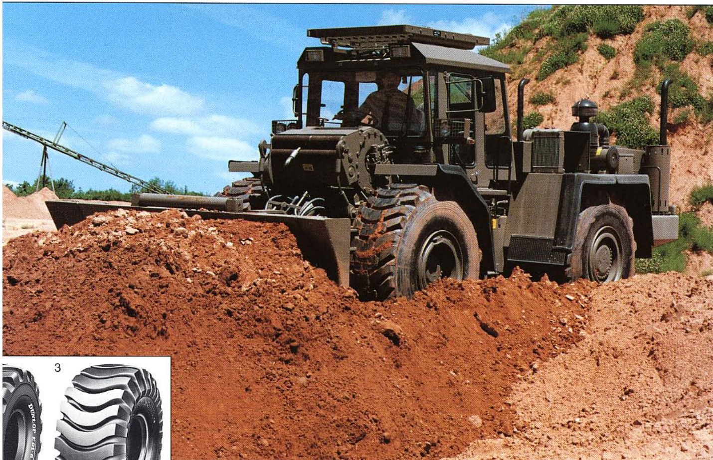
Three tyre types are well-proven for ZM-wheel dozers: the two radial tyres 26.5 R 25 and the diagonal tyre 30/65-25 16 PR.
