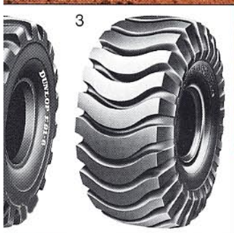
Three tyre types are well-proven for ZM-wheel dozers: the two radial tyres 26.5 R 25 and the diagonal tyre 30/65-25 16 PR.
