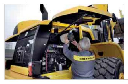
The W190B is designed for simple and easy maintenance and service procedures thanks to its excellent ground level access to all the most important components and to the new high-tech digital display located on the dashboard, which keeps the operator fully aware of all machine main functions, such as engine and transmission diagnostics, error reporting and warning prompts.
