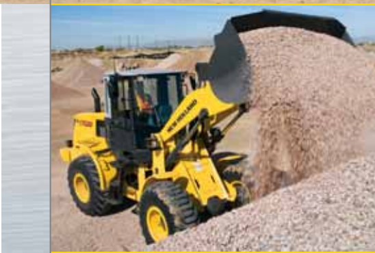
New Holland Z-linkage loader design delivers outstanding breakout force.
