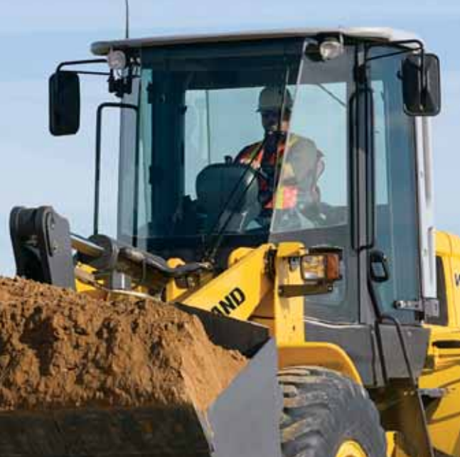
Flat glass provides an unobstructed view to the bucket and the worksite.
