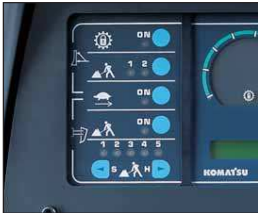
Track shoe slip control panel
