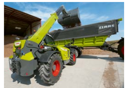
The weighing system also allows accurate filling of road transport vehicles
