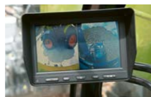
The images from the front and rear cameras are transferred to the monitor in the cab
