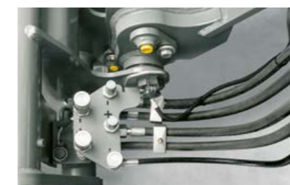
Hydraulic connections in a well-protected location on the implement carrier
