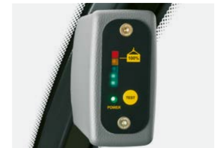
Load display based on clear traffic light system: When the stability limit is exceeded, all the LEDs light up, and an alarm tone sounds
