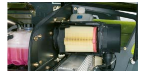
The engine air filter is very readily accessible, with no tools required for maintenance
