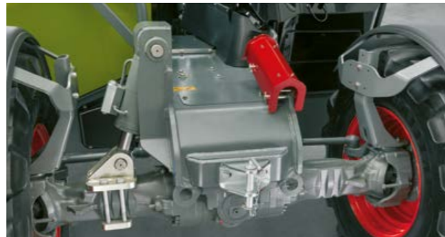
Greater off-road safety through hydraulic levelling function
