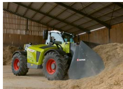
Automatic bucket return for fast working close to the ground
