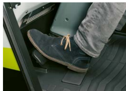
The brake with inching function reduces fuel consumption and brake wear
