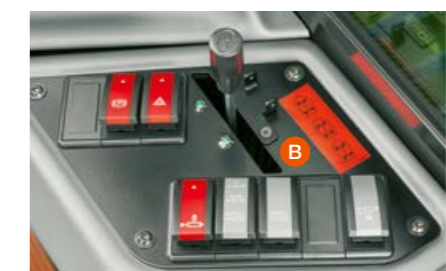
Control lever (B) for adjusting the steering mode in the basic class
