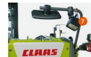
Halogen lights on the rear-view mirror bracket for illuminate the rear area
