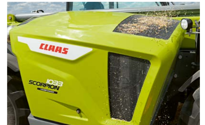
Minimum radiator soiling, thanks to the reversible fan
