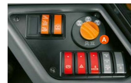
Push and turn switch (A) for selecting the steering mode in the SCORPION VARIPOWER
