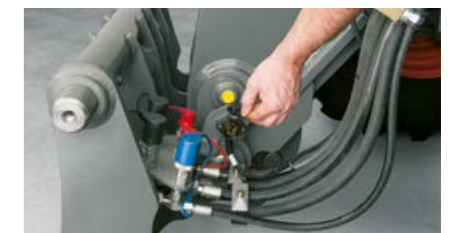
Sockets for flexible power supply for wide range of attached and trailed implements
