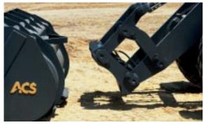
**Hydraulic Quick Coupler** — For quick and easy attachment changes, the optional hydraulic quick coupler saves time and boosts productivity.
