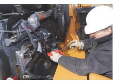
Ground-level fluid checks make daily maintenance quick and easy.
