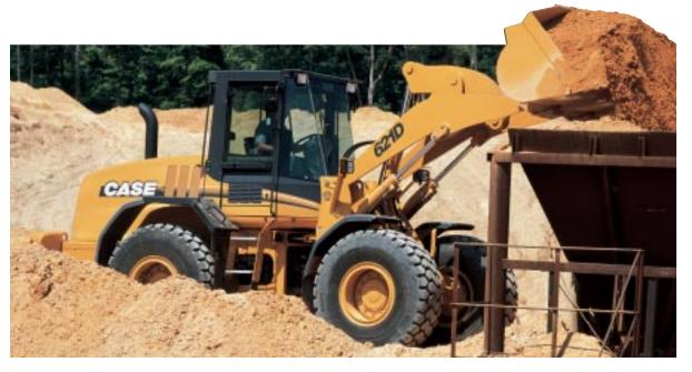
Newly designed D Series buckets more efficiently slice into the pile and fill more quickly and fully than ever before. The new bolt-on cutting edge has been redesigned to penetrate the pile like a knife.
