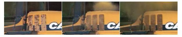
In work environments with high levels of dust or airborne debris, the D Series optional reversible fan provides a time-saving solution to cleaning the cooling module.
